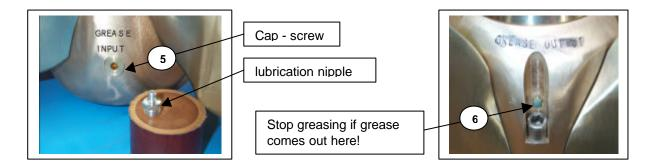
Factory supplied special grease EP/SAL is recommende and available from your VARIPROP distributor. **Avoid regular white grease (sterntube-grease)!**
