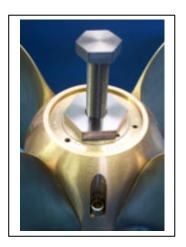
**4.)** Now screw the hexagonal head bolt into the nut and turn the bolt against the shaft until the VARIPROP comes off the taper. Never use a hammer to remove the prop from the taper !
