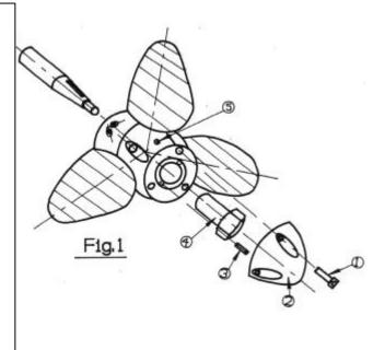
**MOUNTING:** First slide the prop on the shaft without key. Mark the shaft with a grease-pen at the prop end. After tightening the shaft nut very strongly (torque-setting see page 9) the mark must disappear. If not, the key is binding and the top or the sides of the key must be filed down. Light must be shining through on the top of the key when looking into the hub from astern. You may have to move your eye vertically to see it.
