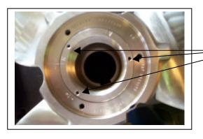
Only two of the three lock-pin holes can be used, depending on the  $\frac{\text{final position}}{\text{of the shaft-nut flange ( 3 )}}$ .
