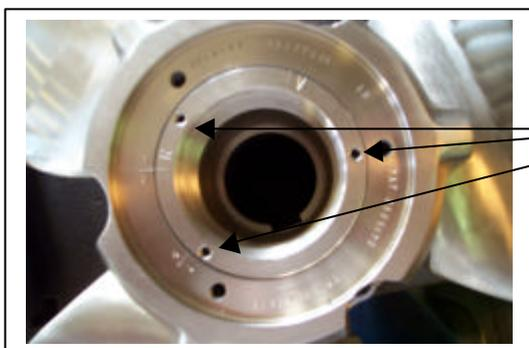
**Only two** of the three lock-pin holes can be used, depending on the final position of the shaft-nut flange ( 3 ).
