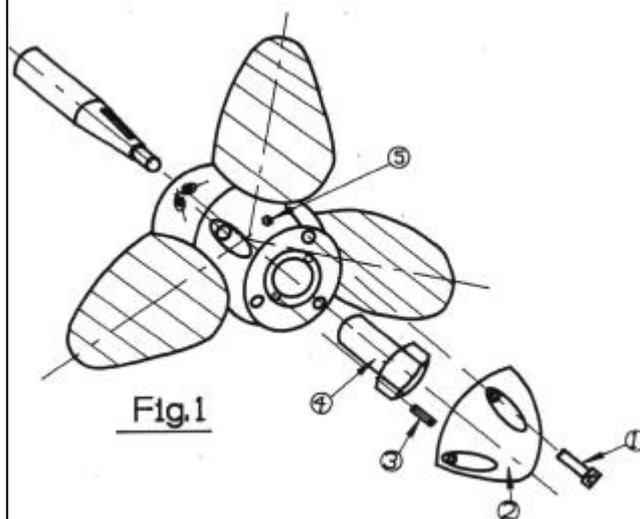
**MOUNTING:** First slide the prop on the shaft without key. Mark the shaft with a grease-pen at the prop end. After tightening the shaft nut very strongly ( torque-setting see page 9 ) the mark must disappear. If not, the key is binding and the top or the sides of the key must be filed down. Light must be shining through on the top of the key when looking into the hub from astern. You may have to move your eye vertically to see it.
