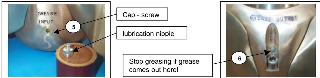
Factory supplied special grease EP/SAL is recommended and available from your VARIPROP distributor. **Avoid regular white grease (sterntube-grease) !**
